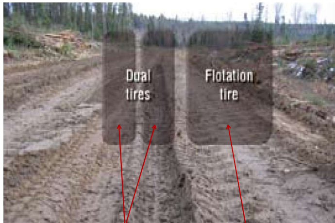
Dual application of Conventional truck tires
